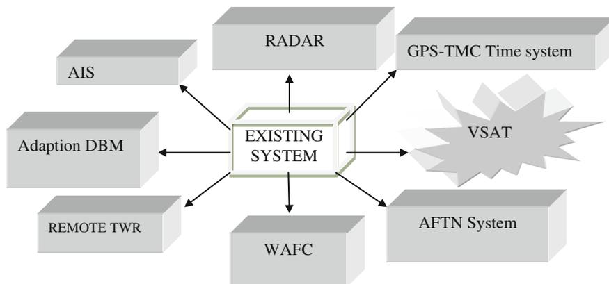
**Fig. 52.1** The architecture of existing flight communication system
