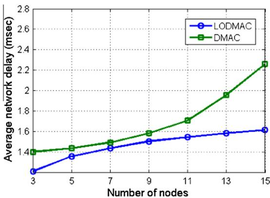
Fig. 9. Average network delay of LODMAC and DSMAC protocols.
