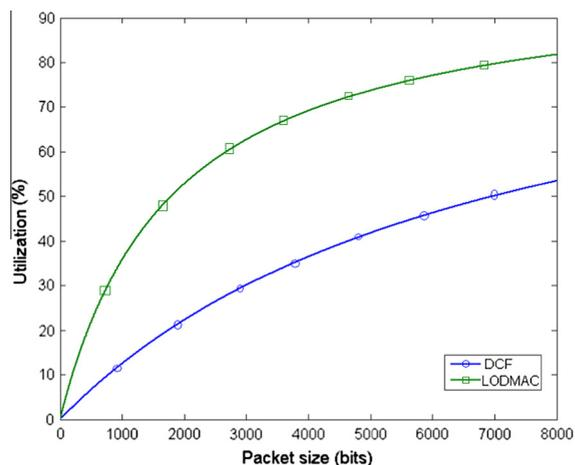
Fig. 4. With two transceivers on nodes, the wireless channel is utilized more effectively.
