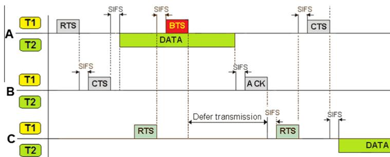
Fig. 7. Communication control sequence with BTS packets.
