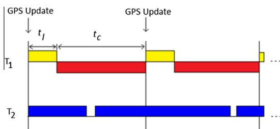
Fig. 1. LODMAC sequence with a pair of transceivers.
