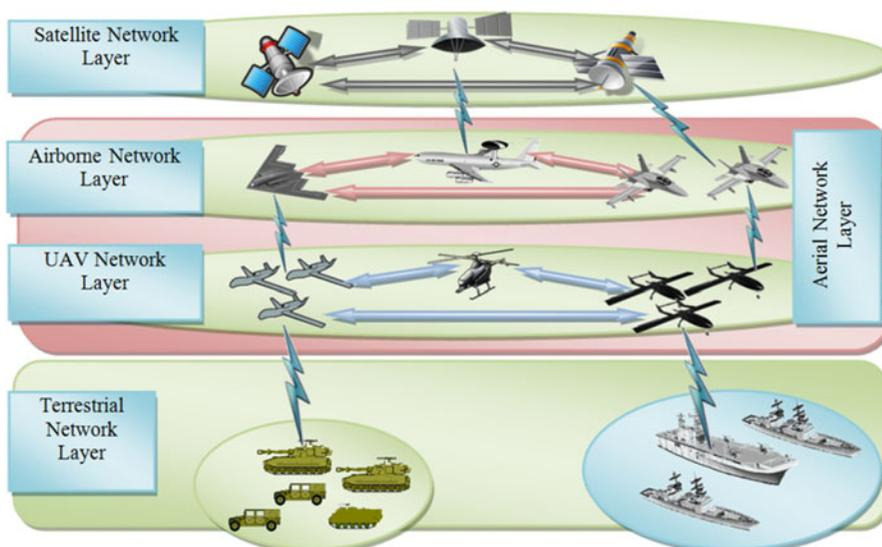
some routing protocols have been proposed for FANETs. These protocols mainly depend on communication types. In a FANET, there are mainly two different communication types: *UAV-to-UAV* and *UAV-to-Infrastructure communications*.
